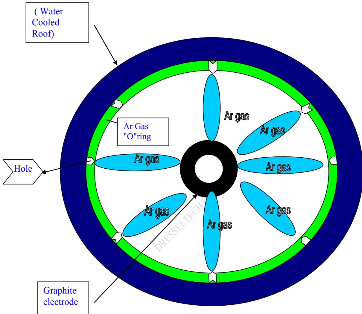
This figure shows cross-section of the "O"ring with Ar gas blowing mounted to the water cooled roof .
