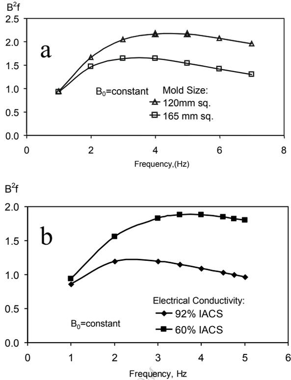
Fig 1. Effect of the mold size (a) and electrical conductivity (b) on magnetic torque.
